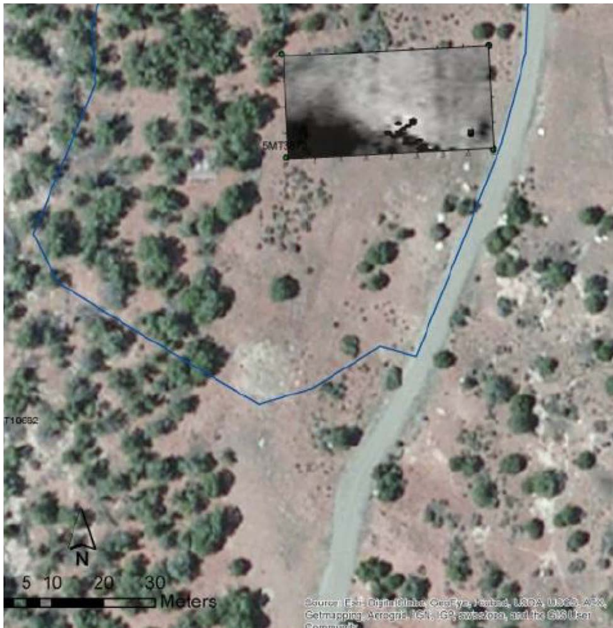
Figure 3.36. Aerial photograph of Site 5MT3873 overlain with the electrical resistance results and the site boundary (blue).
