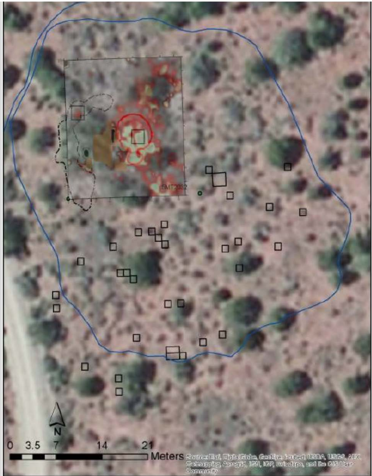
Figure 3.35. Aerial photograph of Site 5MT2032 overlain with electrical resistivity results, pithouse orientation (red), roomblock outline (dashed line), excavation units (black), and site boundary (blue).
