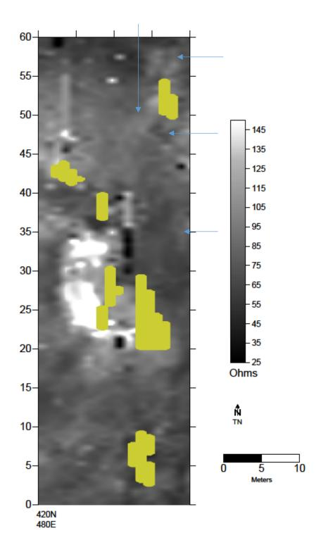
Figure 22. Electrical resistance survey conducted during 2018 of Grids 1, 2, and 3, the Haynie site. Yellow indicates dummy values, and blue arrows point to areas of interest for further investigation. Image created by Mona Charles, Powderhorn Research LLC, 2018.
